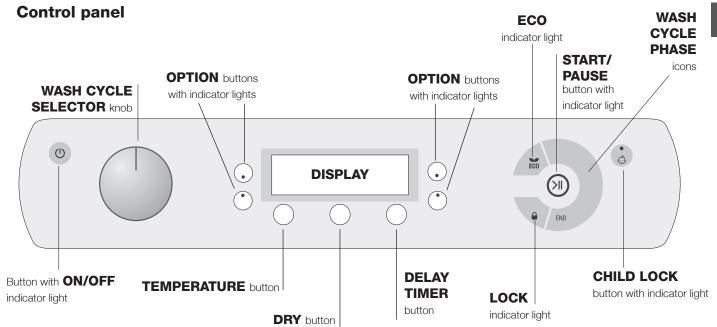
Button with () **ON/OFF** indicator light: press this briefly to switch the machine on or off. The green indicator light indicates that the machine is switched on. To switch off the wasdher-dryer during the wash cycle, press and hold the button for approximately 3 seconds; if the button is pressed briefly or accidentally the machine will not switch off. If the machine is switched off during a wash cycle, this wash cycle will be cancelled.
